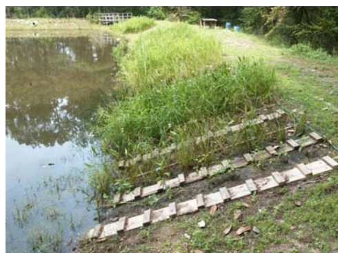
Fig. 1 Photograph of the experimental wetland, showing lanes of monocultures of plants grown on a shoreline graded to a 33 % slope (photo credit: Randy Bergeron)
